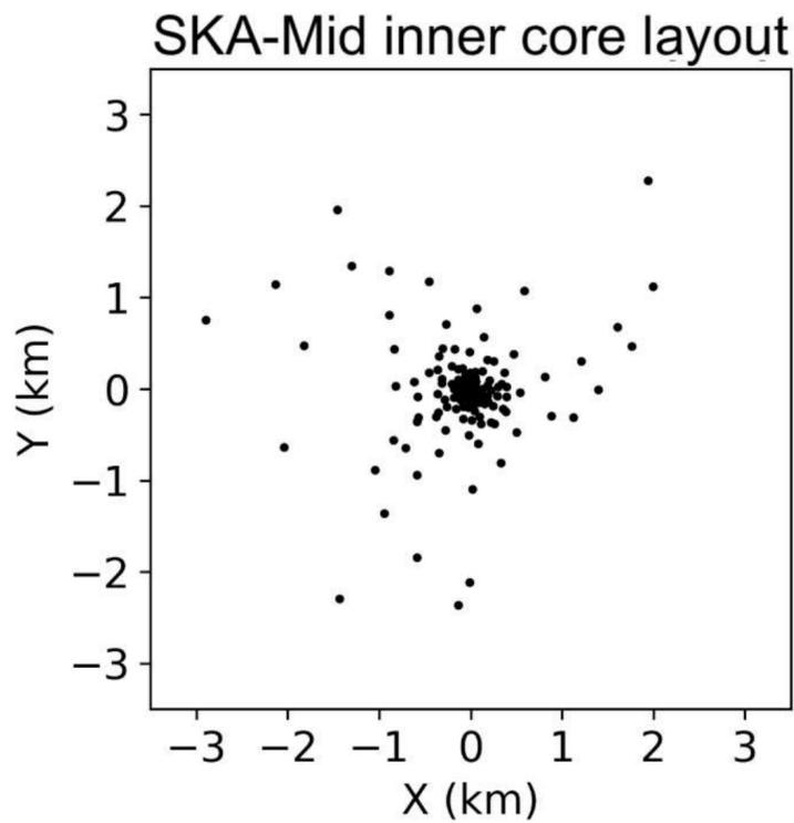
Layout of the inner core of SKA-Mid. The figure show the core and the first few dishes in the spiral arms. The dots represent individual dishes.
