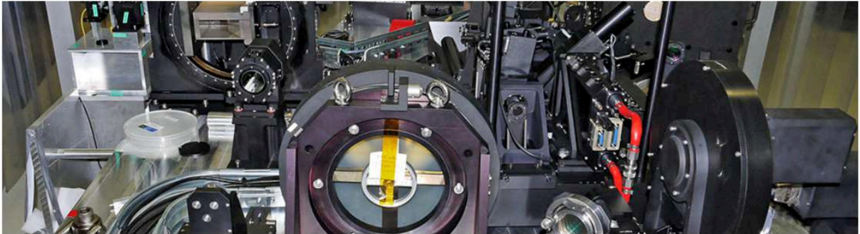
IRDIS: InfraRed Dual-band Imager and Spectrograph.
