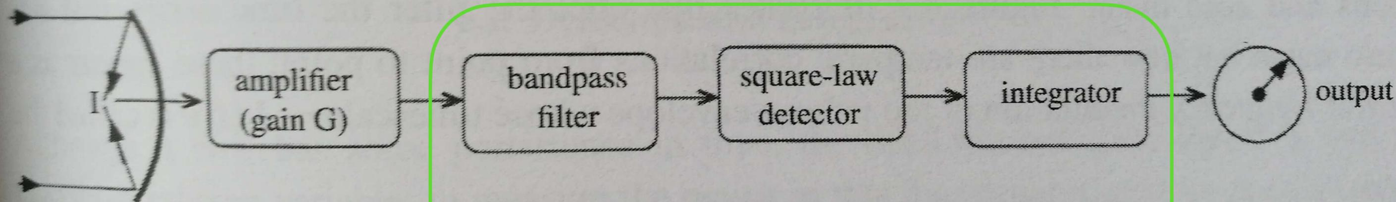
Figure 6.1. The basic components of a linear radiometric receiver.
